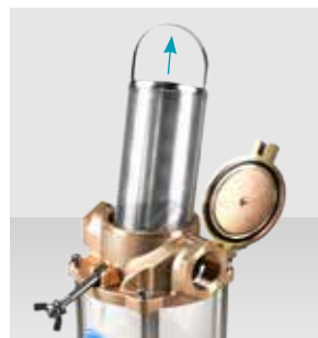
3 Pull out the stainless filter
